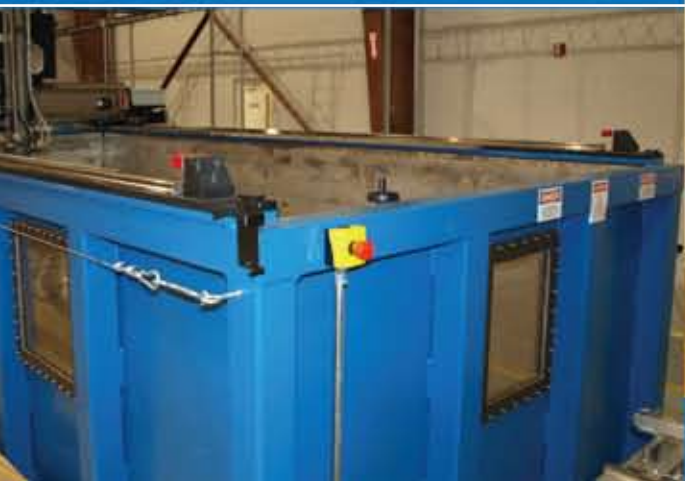
Phased Array instrumentation with Contour-Following immersion inspection capabilities.
