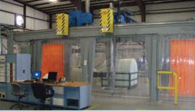
Large Complex-Contour Scanning Gantry with 1 & 5 MHz Dual PE and TTU
